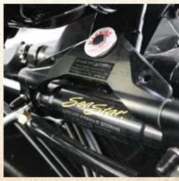
**SEA STAR® HYDRAULIC STEERING**OPTIONAL | maximum steering control and comfort suitable for use with high-performance propellors and jack plates
