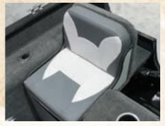
FLIP-UP JUMP SEAT OPTIONAL Convert from a spacious casting deck to additional passenger seating at the stern.
