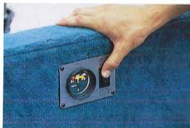
Battery charge switch
